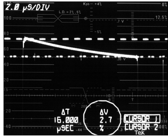
Figure 34. The 1780R voltage and time cursors can facilitate line time distortion measurements.
